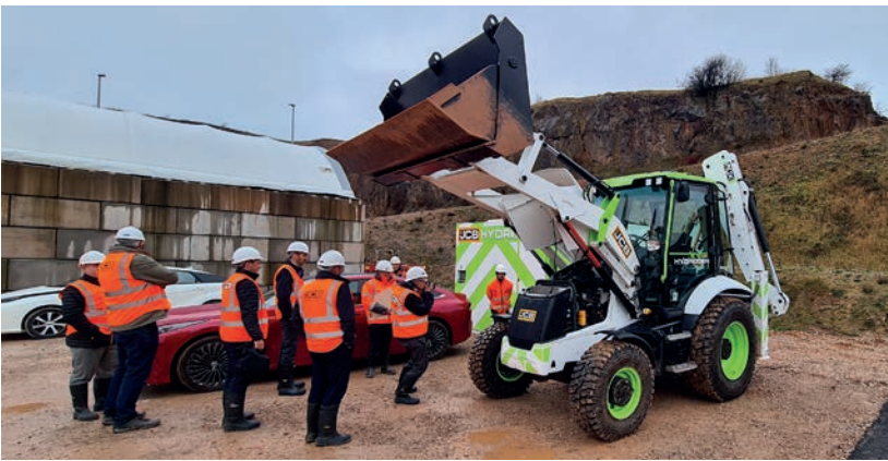
JCB backhoe fitted with hydrogen internal combustion engine
