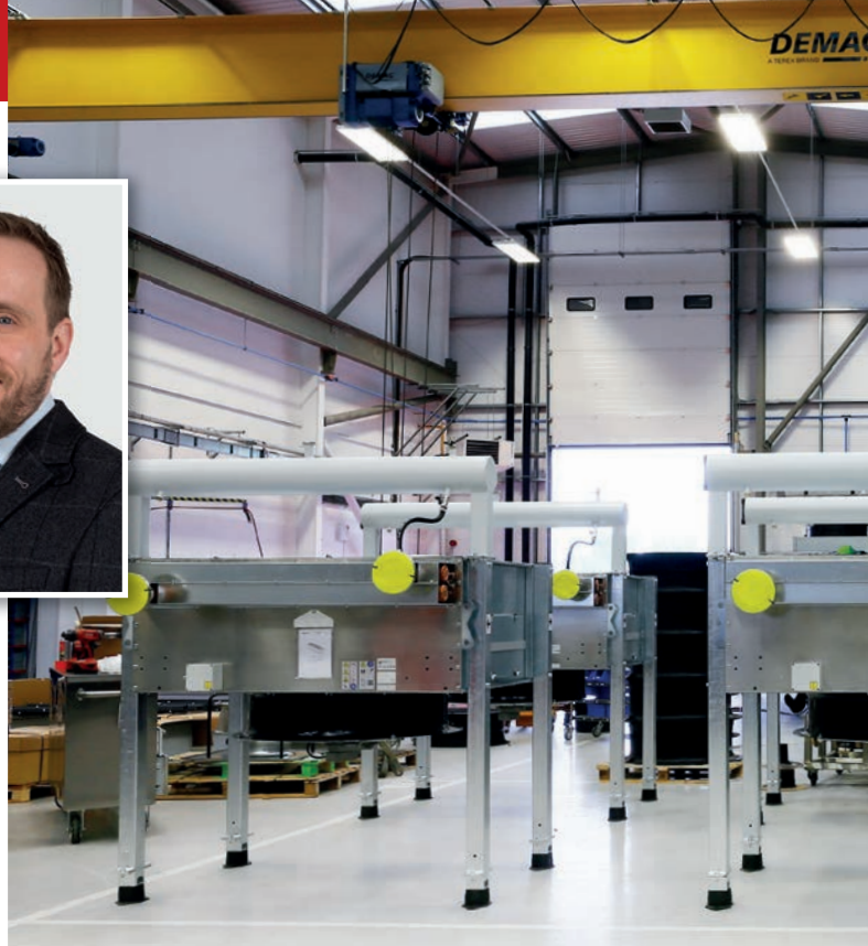
Gen set coolers with header tanks
